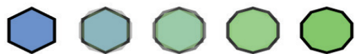
Fig. 2. Principle of alpha blending, transitioning from a low quality model to a high quality model
