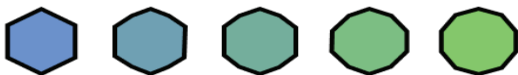
Fig. 4. The principle of geomorphing, going from a low quality model to a high quality model
